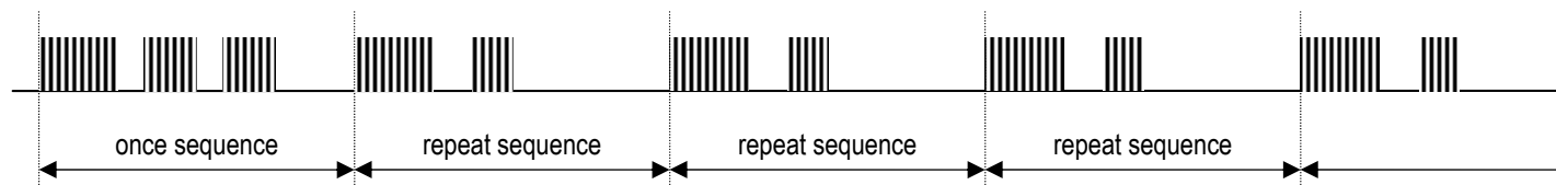
Picture 3: Cutting IR signal into once sequence and repeat sequence
